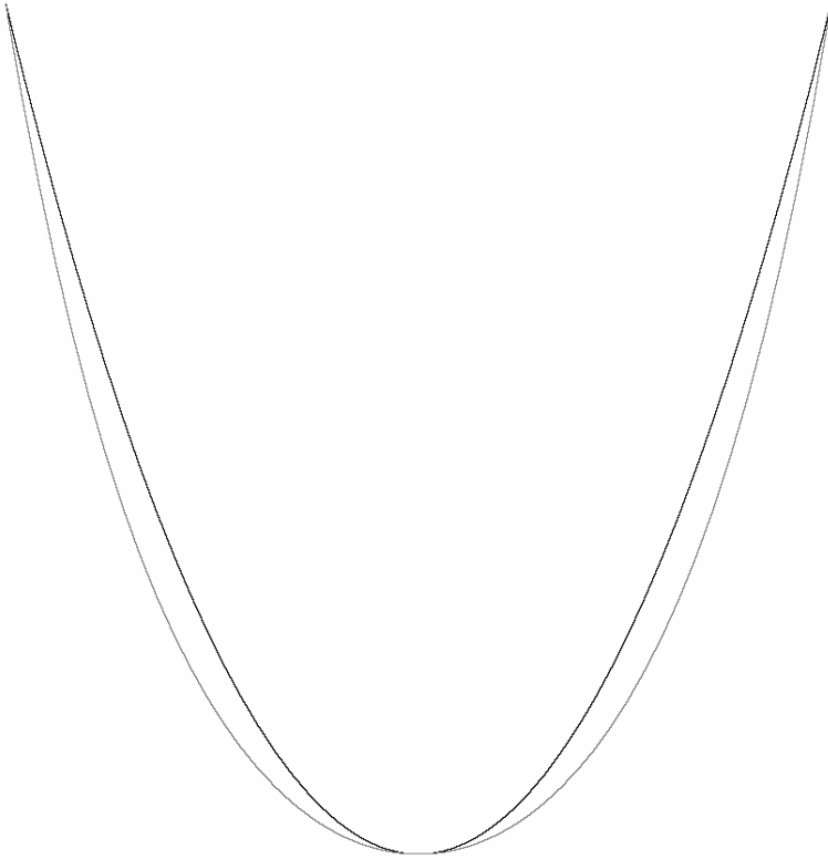
Fig. 3. Parabola and Catenary with aspect ratio 1:1
